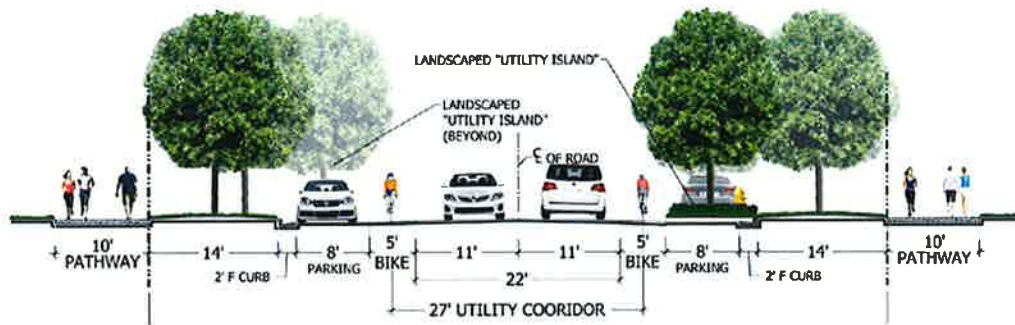
TC-1 | TTD COLLECTOR WITH ON STREET PARKING
