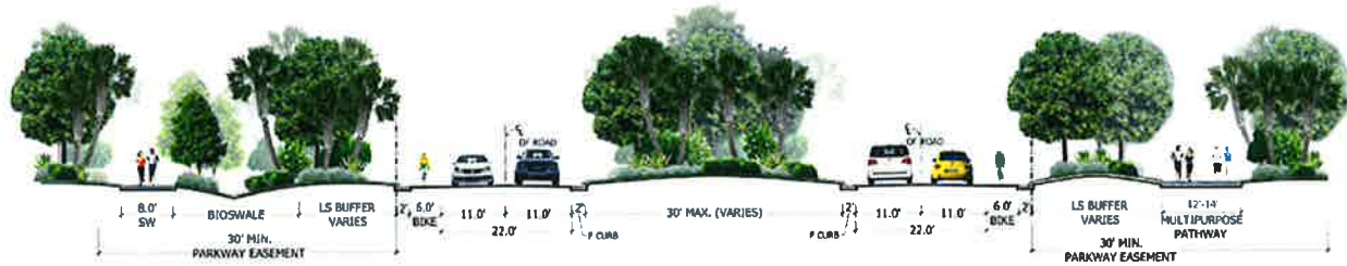
C-7 | 4 LANE DIVIDED TTD COLLECTOR ROAD WITHOUT ON STREET PARKING 45 MPH
