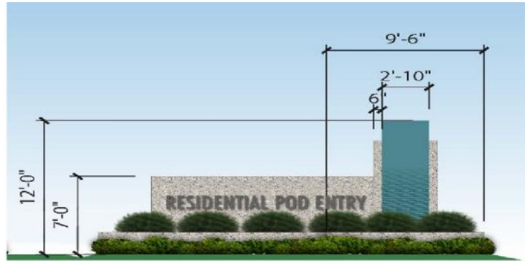
Figure 6-4: Residential Pod Entry Monument
