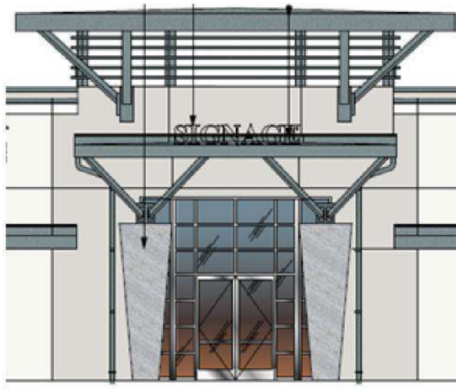
Figure 6-7: Ground Floor Permanent Canopy Sign
