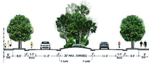
C-9 | 2 LANE DIVIDED TTD COLLECTOR ROAD WITHOUT ON-STREET PARKING 45 MPH (* 8' SIDEWALK MAY MEANDER OUTSIDE OF ROW, SUBJECT TO PED EASEMENT.)
